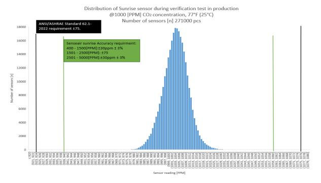
2- Senseair Sunrise sensors accuracy test based on the latest addition, Addendum ab, to the ANSI/ASHRAE Standard 62.1-2022: Tested CO₂ concentrations are 400, 600, 1000, 1500, 2000 and 2500 [PPM] at temperature 77°F (25°C). All sensors are within the updated Addendum ab, to the ANSI/ASHRAE Standard 62.1-2022 (accuracy of ±75[PPM] at 600, 1000 and 2500 [PPM] CO₂ concentrations).
